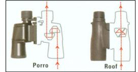
**Roof prisms** binoculars have straight tubes (the objective lens is in line with the ocular lens), and they are therefore more compact and easier to hold properly for birding. Roof prism binoculars are typically better sealed against dirt and moisture and are of more rugged construction because most moving parts are internal.
